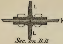
Fig. 190 B—Is a section on the line D D of Fig. 190. K is a vertical side plate. L L are angle irons which are riveted to the side plates.
